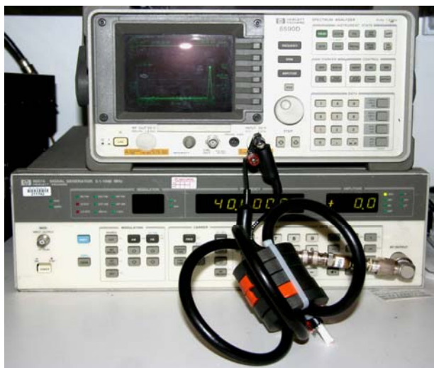
Fig 40a – Measuring Coaxial Chokes
