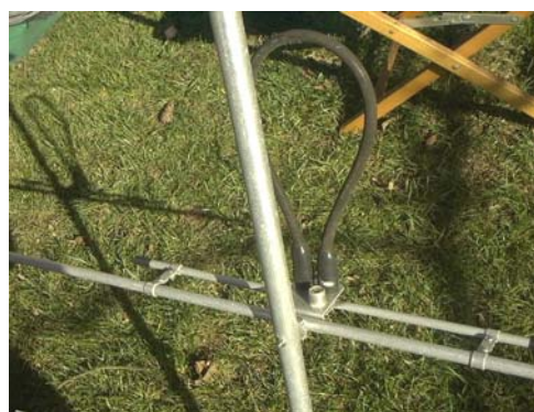
Fig 32 – A Half-Wave Balun
