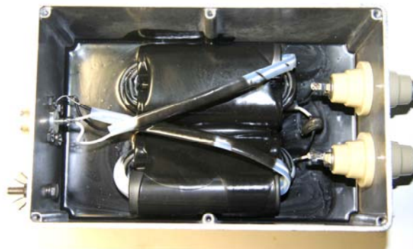
Fig 38 – Current Choke (Guanella) Transformer
