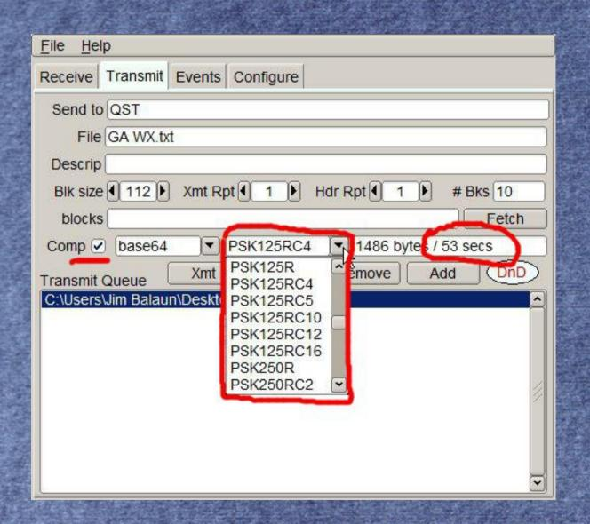
Make sure the automatic interface between FLDIGI and FLAMP made the switch to the selected mode and that the bandwidth is not interfering with another station on the waterfall.
