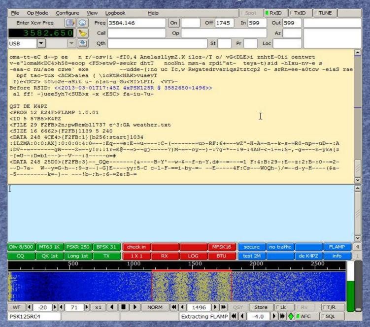
In this case only 1 of 5 blocks had the proper checksum so the receiving station will need to Report (when asked) which will put the missing files need in the transmit screen on FLDIGI. You must then start and stop transmission on FLDIGI.
