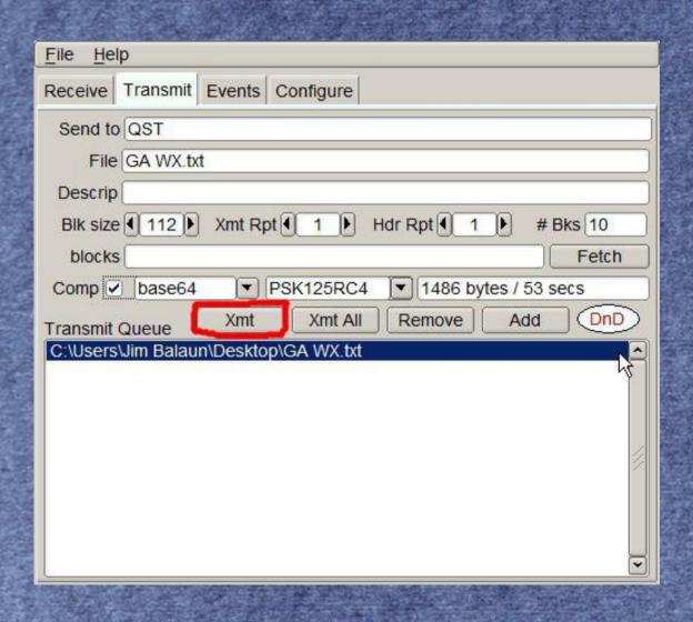
Reselect the mode or try others to get the time reasonable. Reliability will be reduced with higher speeds and a wider bandwidth will likely cause interference on the frequency in use. Reselect even if the mode you plan to use is already in the box. Select Comp for compression.
