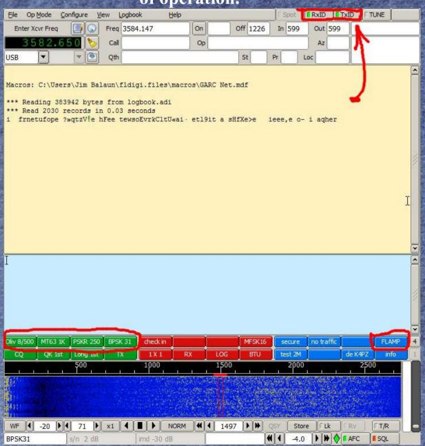
Start FLAMP, "drag and drop" your text file to the spot indicated on the Transmit screen. The file will automatically copy to the Transmit Queue.
